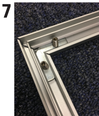
7 Place screws into the joiner pieces.
