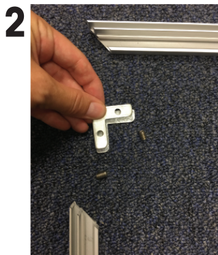
2 Place joiner piece with holes on top of solid joiner piece.
