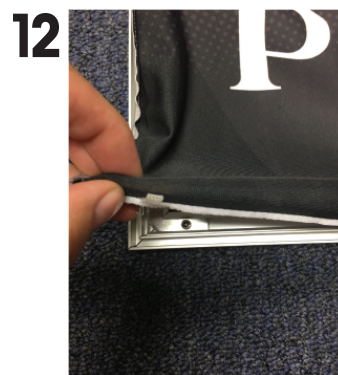
12 Fold edge and insert into outermost extrusion channel.
